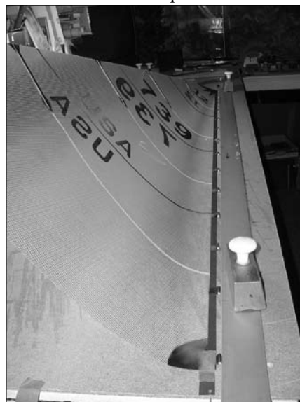
Photo 2: Main luff measurement.
